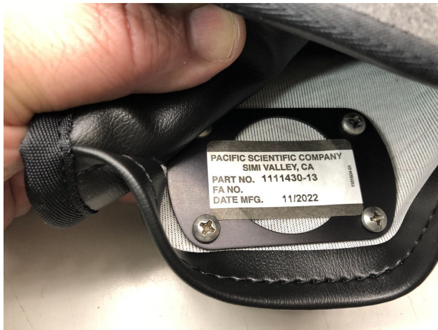
Figure 2 Rotary Buckle DOM Location with Buckle Pad
