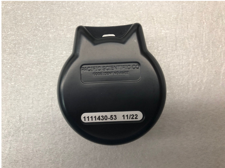
Figure 3 Rotary Buckle DOM Location without Buckle Pad
