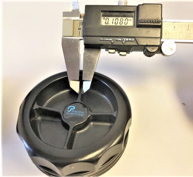
Figure 3 Correct Buckle Measurement
