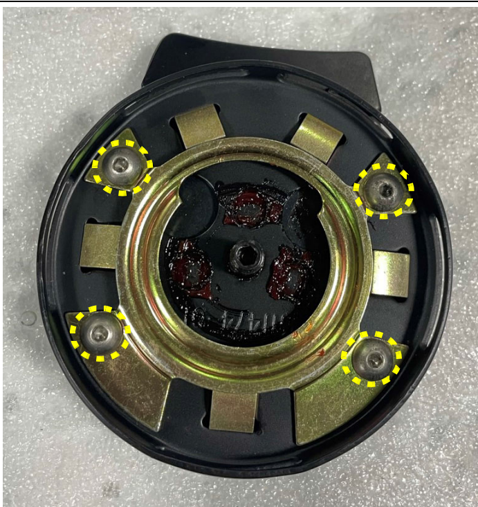
Figure 13 Disassembled Rotary Buckle with Suspect Torx Head Screws
