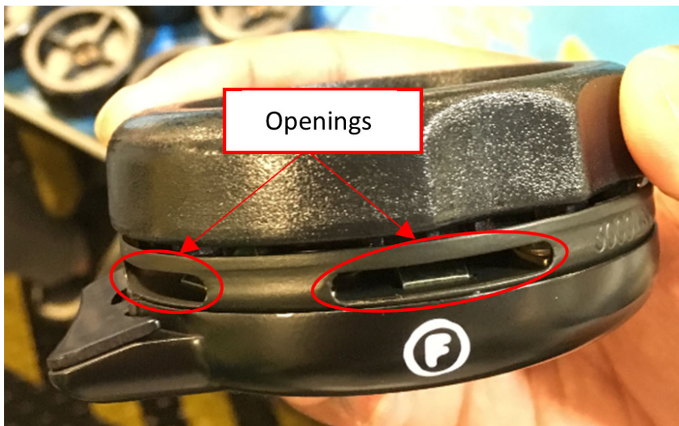
Figure 4 PNR 1111475 Series Rotary Buckle Openings for Inspection
