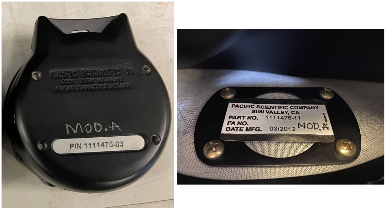
Figure 15 Re-Identified PNR 1111475 Series Rotary Buckle Assembly with “MOD. A”
