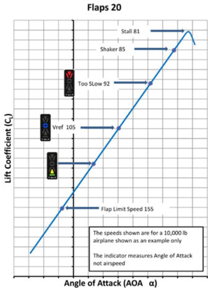
Figure 1 Lift Coefficient vs AOA
