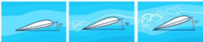
Figure 1: Wing Flow Separation at Stall
